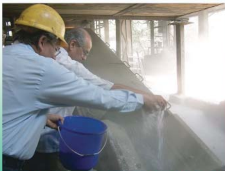
Mixing of plastics waste with stone –Asphalt Plant, BMC
